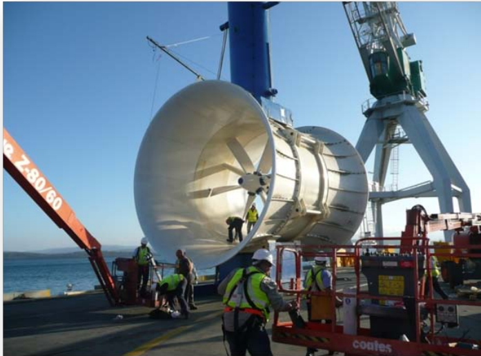
Figure 3: Atlantis' technology Solon ©. Example of horizontal axis energy translation and device fixed to the seabed.
