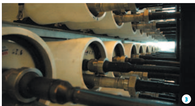
1: The prototype at Tofte, south of Oslo. 2: Water is filtered to avoid clogging of the membranes. 3: Membranes are coiled up inside pressure vessels. 4: The pressure is utilised in a turbine to generate electricity.
