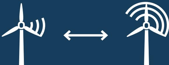
The remote-controllability of wind power plants means they can be controlled in a demand-based way. If there is a high drop in demand, plants are slowed down or stopped temporarily. When demand increases they are immediately switched on again.
