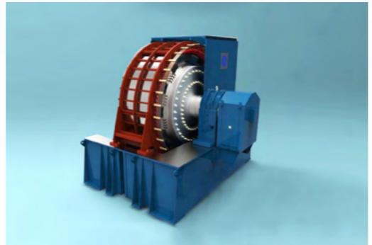
with a large mass to create as much inertia as possible. A rotating stabilizer can also generate and absorb reactive power and provide a large amount of short circuit current during transmission network faults, which helps with stabilizing the local voltage level during steady state and fault conditions. Statkraft is building two rotating stabilizers at Keith in Scotland, and this is scheduled for completion in the autumn of 2021.
