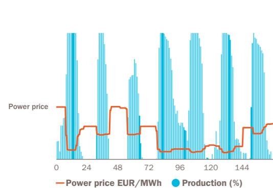
Hydrogen production is flexible. Statkraft's analyses show that in the future, electrolyzers will tend to run during the day. The graph to the left shows green hydrogen production during a week compared to the power price and the graph to the right shows the average hourly production of green hydrogen compared to the average power price throughout the day
