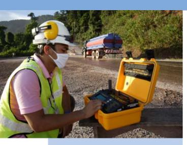
ABOVE: Dust monitoring along roads and near construction sites to ensure compliance to international standards FACING PAGE: Waste management facility, from where many items are recycled
